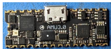
Figure 5: AMU used for measuring cell temperature and IV Curves.
